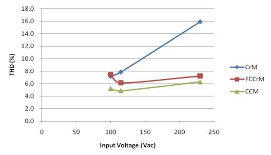
Figure 9–6. Total Harmonic Distortion Comparison
