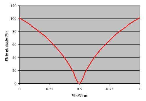
Figure 6-4. Peak-to-Peak Ripple of the Input Current as a Function of the Line Magnitude
