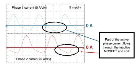
Figure 7–6. Part of the Current Flows through the Supposedly Inactive MOSFET and Coil
