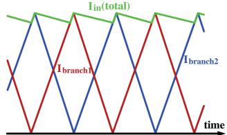
Figure 6–3. The Total Current Exhibits a Reduced Ripple
