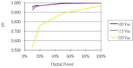
Figure 3–9. Power Factor Performance Over Line and Load
