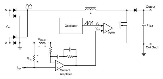
Figure 1–18. Diagram for Average Current Mode Control Circuit
