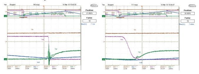
Figure 4–7. Turn–On Waveforms with (Left) No ZCD Delay and (Right) Optimized ZCD Delay
