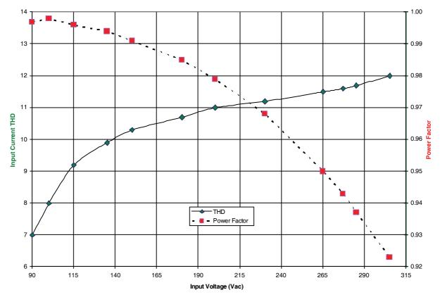
Figure 8–5. THD and Power Factor with 12 LED (Vf = 37 Vdc) Load Over a Wide Input Range
