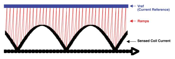
Figure 1–21. Predictive CCM Control Waveforms
