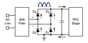
Figure 7–1. The Input Current Flows Through Two Diodes
