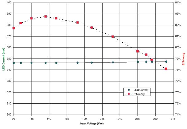
Figure 8–4. Line Regulation and Efficiency Driving 12 LED Load (Vf = 37 Vdc)
