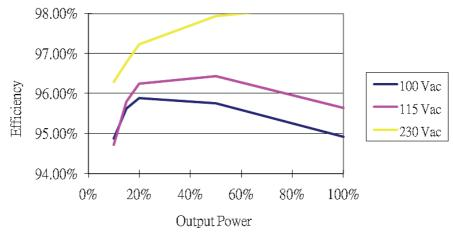
Figure 3–8. Efficiency Performance Over Line and Load
