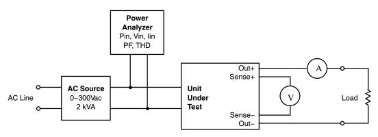
Figure 2–5. Test Set–Up for Performance Measurements
