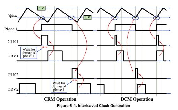
As a voltage mode controller, the NCP1631 forces the MOSFET on-time to be identical in both branches. The demagnetization time that only depends on the conduction time and on the line and output voltages is then the same in both
