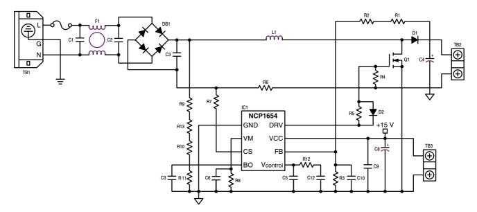
Figure 5–3. Circuit Schematic of the CCM PFC Circuit Based on NCP1654
