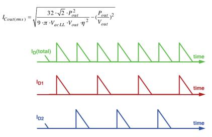
Figure 6–5. Reduction in the AC content of the Refueling Current as a Result of Interleaving
