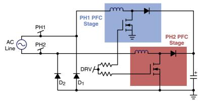
Figure 7–3. Two–Phase Architecture
