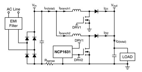
Figure 6–2. Simplified Schematic of an Interleaved PFC Stage
