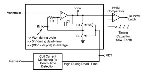
Figure 4–2. DCM PFC Algorithm to Modulate on Time
