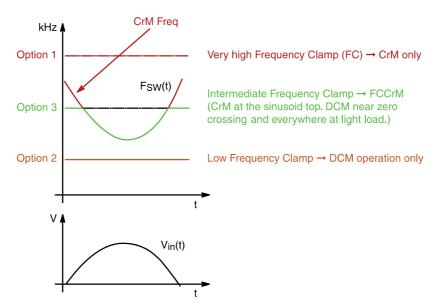
Figure 1–16. PFC Mode Selection Through Frequency Clamping
