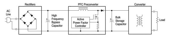
Figure 1–4. PFC Preconverter Stage
