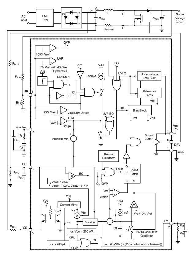
Figure 5–1. NCP1654 Block Diagram
