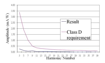
Figure 5-4. Harmonic Spectrum of the 270 W CCM Converter
