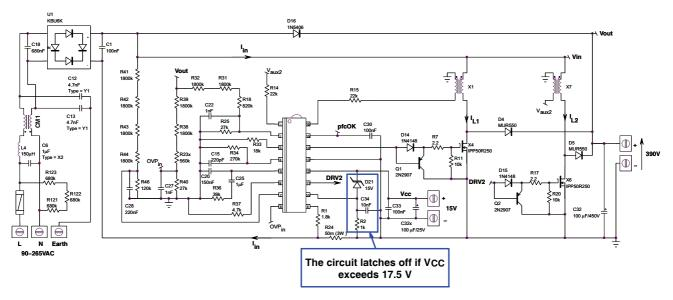
Figure 6–7. Application Schematic
