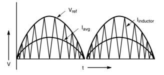
Figure 1–9. CRM Waveforms
