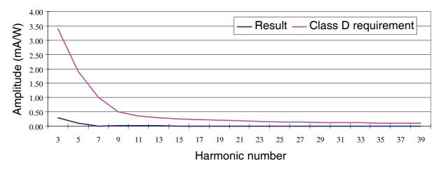
Figure 4–5. Harmonic Spectrum of 270 W FCCrM Converter at Full Load
