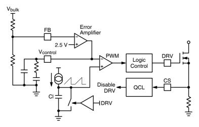
Figure 1–11. Simplified Schematic of CrM Controller Without Multiplier
