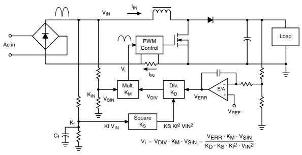
Figure 1–17. Block Diagram of the Classic PFC Circuit
