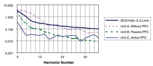
Figure 1–6. Input Harmonics of Three PC Power Supplies Relative to IEC61000–3–2 Limits
