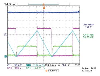
Figure 3–5. Operating Waveforms at Full Load, 115 Vac
