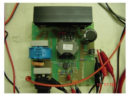
Figure 9–1. Picture of NCP1654 Demo Board Used for Comparisons
