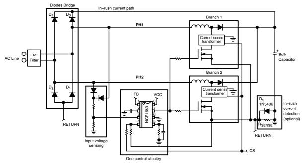
Figure 7–7. Simplified Application Schematic of Bridgeless Converter
