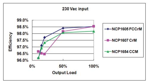
Figure 9–5. Efficiency Performance at 230 Vac
