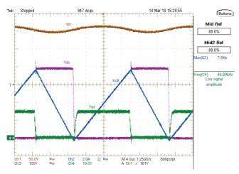
Figure 4–8. Switching Waveforms at Full Load, 115 Vac Input
