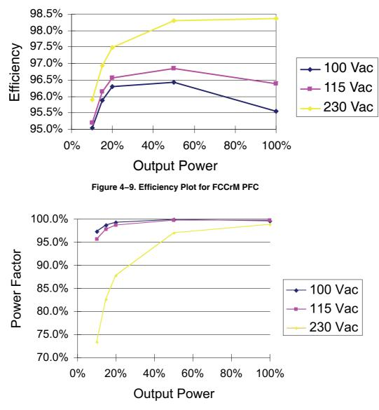
Figure 4–10. Power Factor Plot for FCCrM PFC
