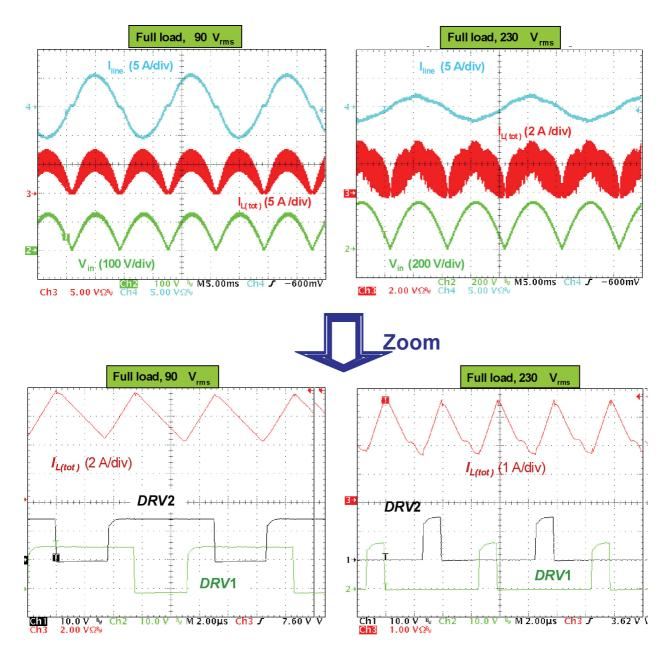
Figure 6–8. Typical Waveforms at full load
