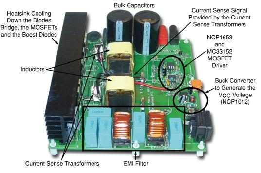
Figure 7–9. Photograph of the Evaluation Board
