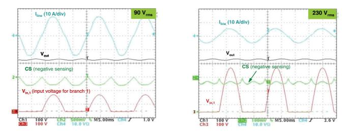
The performance of the board is captured in following waveforms and graphs. Figure 7–11 shows the typical waveforms (line current, output voltage, current sense signal and rectified input voltage) for one branch at two line voltage conditions.
