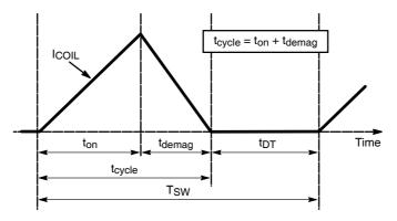
Figure 1–14. DCM Operating Waveforms
