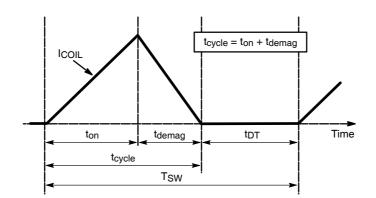
Figure 4–1. States of Operation in Discontinuous Conduction Mode PFC
