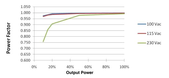
Figure 5–6. Power Factor Performance of the 270 W CCM Design
