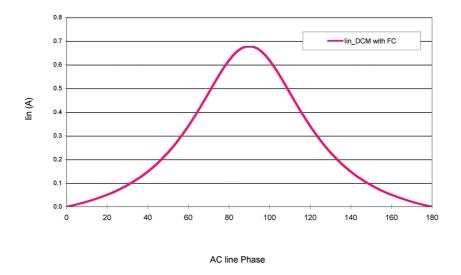
Figure 1–13. CrM Line Current Distortion Due to Frequency Clamping
