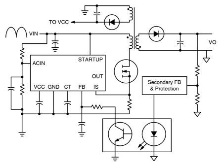
Figure 1–20. Single Stage PFC Using the NCP1651
