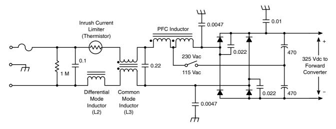
Figure 1–7. Passive PFC in a 250 W PC Power Supply
