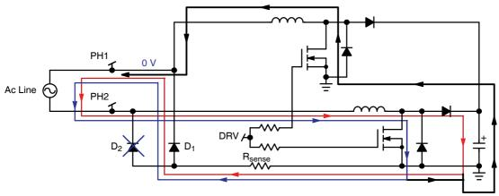
Figure 7–5. Operation for the "PH2" Half–Wave
