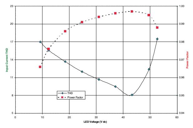
Figure 8–6. Power Factor and THD vs. Load (115 Vac Input)
