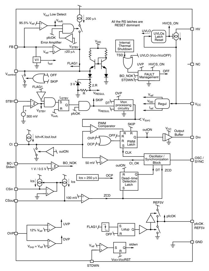
Figure 4–3. Block Diagram
