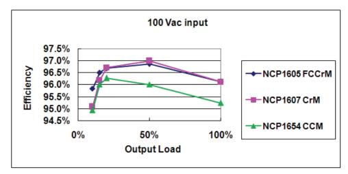
Figure 9–3. Efficiency Performance at 100 Vac
