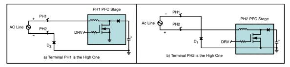
Figure 7–4. Equivalent Schematic for the Two Half–Waves
