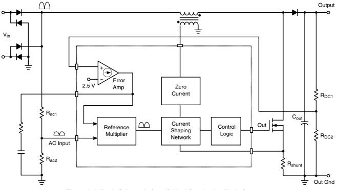
Figure 1–8. Basic Schematic for a Critical Conduction Mode Converter
