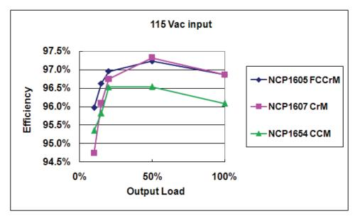
Figure 9–4. Efficiency Performance at 115 Vac
