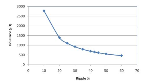
Figure 5–2. CCM Inductance Value as a Function of p-p Ripple
