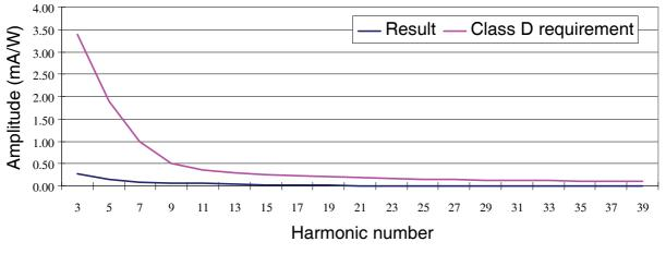
Figure 4–6. Harmonic Spectrum of 270 W FCCrM Converter at 75 W Load
